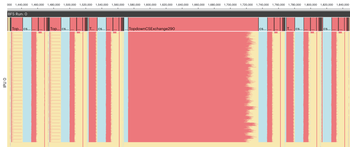
Figure 6.5: Execution profile for a Kron-19-16. Visualizes, how time and resources are spend. The red indicates computation, the blue data exchange, and the yellow synchronization phases.
